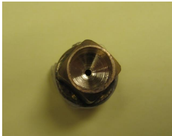
Figure 3. Photograph of the Brass Plug and Orifice, Shown from the Outlet Side
