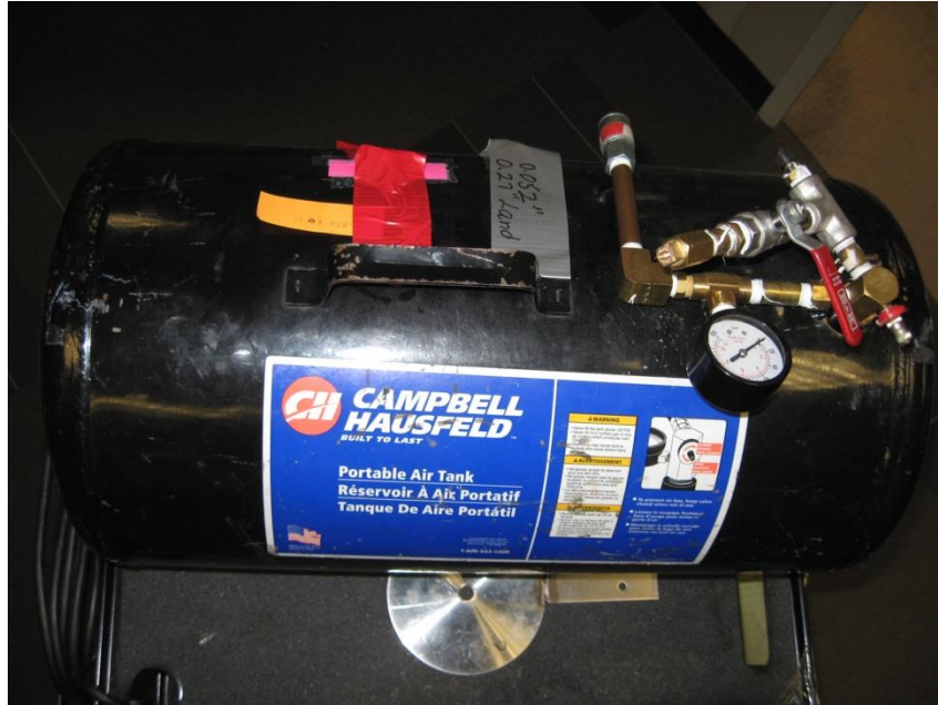
Figure 2. Photograph of the Air Tank and Respective Attachments for Venting Data Collection
